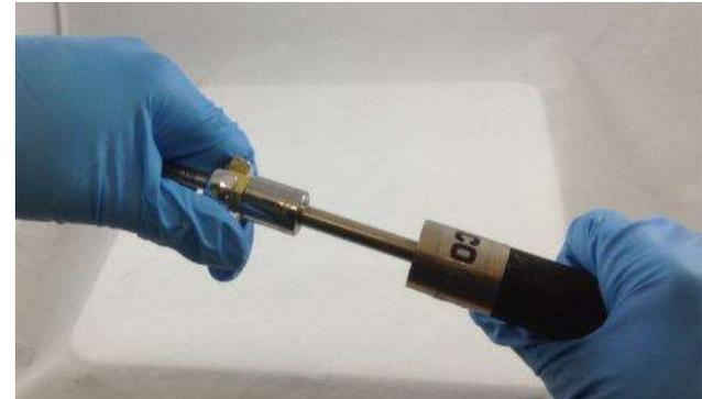
Torque Driver used to tighten Long-term Storage caps
