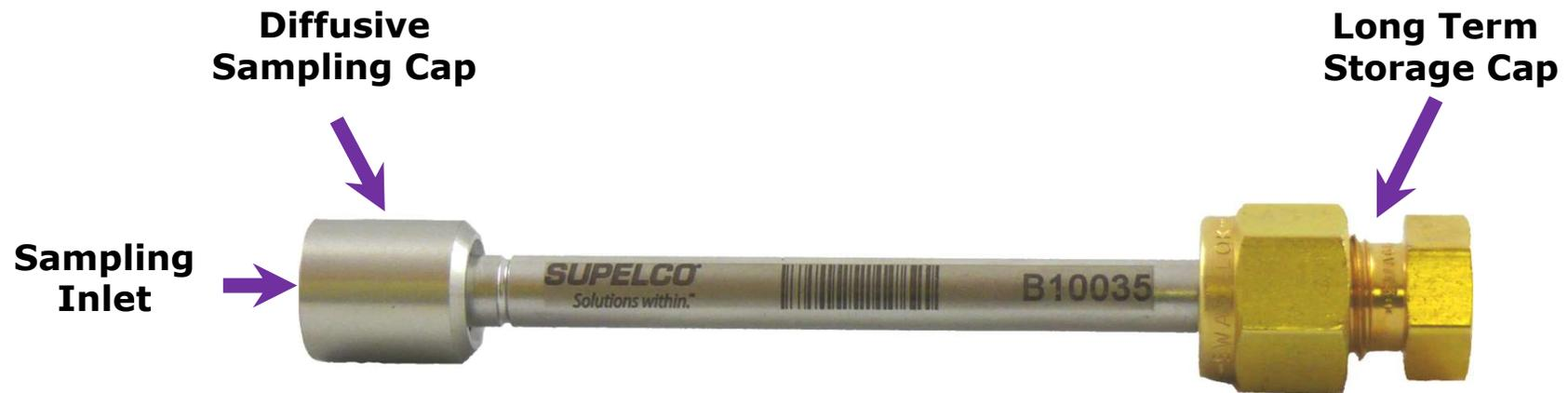
**Tube Dimensions: 3.5-inches (89 mm) long x 1/4 inch (6.4 mm) O.D. x 5 mm I.D.**
